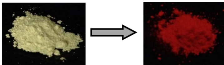
Figure 1: Compound when exposed to visible light (on the left), and to UV light (on the right).
