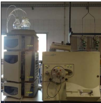
Figure 1: Liquid chromatograph coupled to mass spectrometer.
